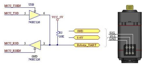
The power is supplied to the CDS55xx servo from the main controller through Pin 1 and Pin 2 of the Molex3P connector.
